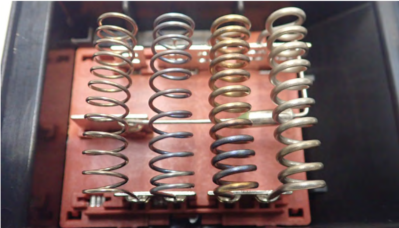
Fig. 3: Controller overloaded due to defective fan
