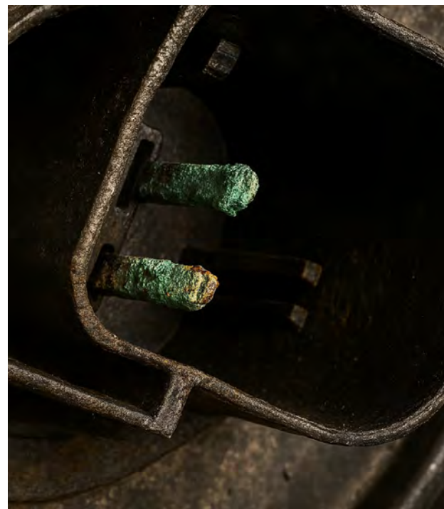
Fig. 2: Corrosion on plug connection
