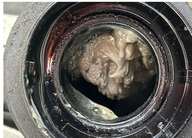
Fig. 2: Oil-in-water emulsion
