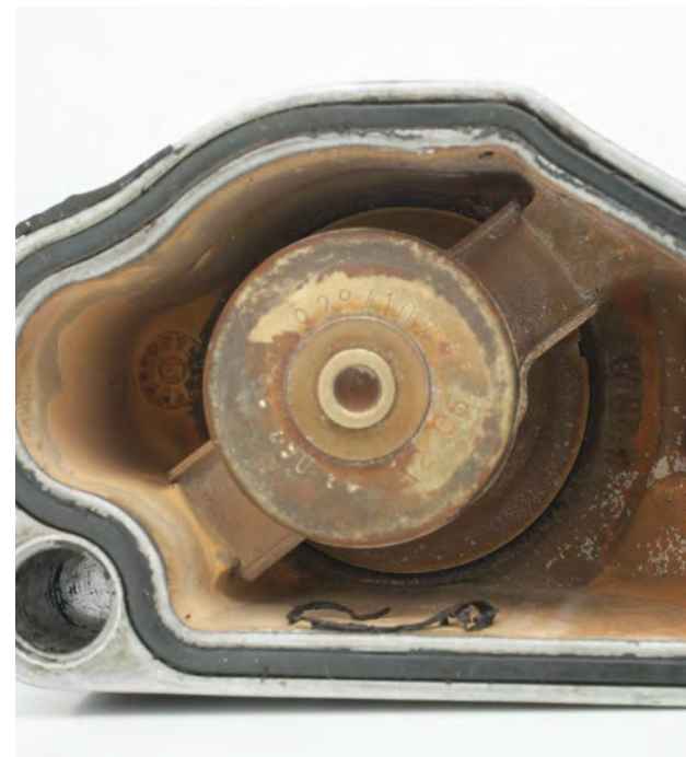
Fig. 2: Corrosion on thermostat
