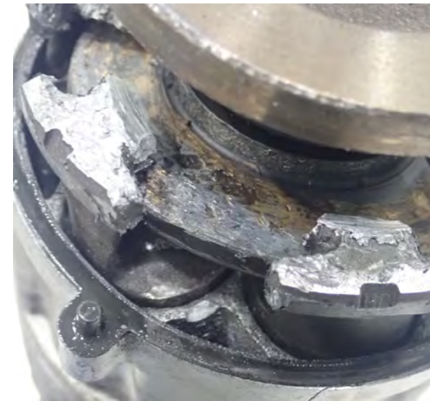
Fig. 3: Seizure marks on pistons and swash plate
