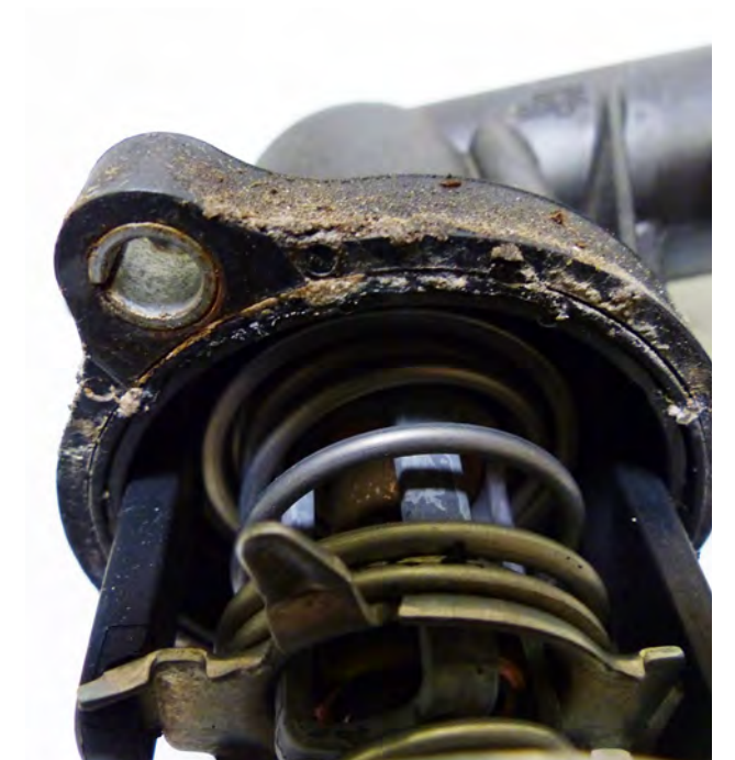
Fig. 2: Seal damaged by additional sealing compound
