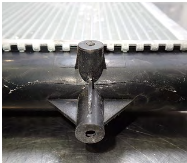
Fig. 2: Burst water tank
