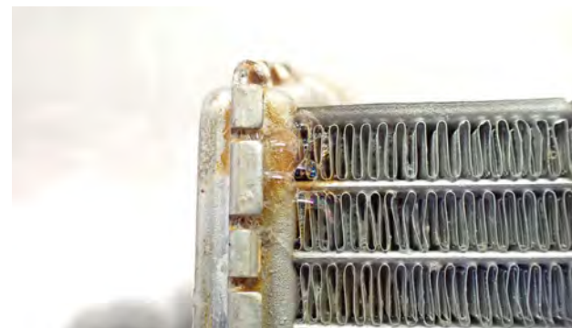
Fig. 4: Corroded heat exchanger
