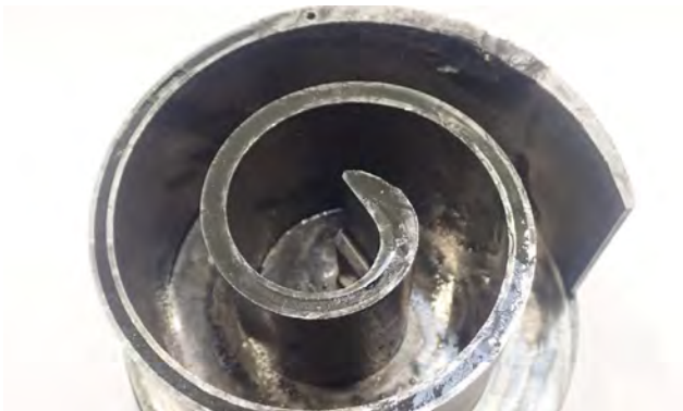
Fig. 1: Scroll in scroll compressor heavily worn
