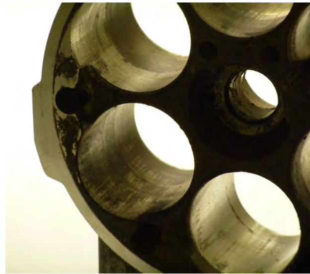
Fig. 2: Seizure marks on the cylinder
