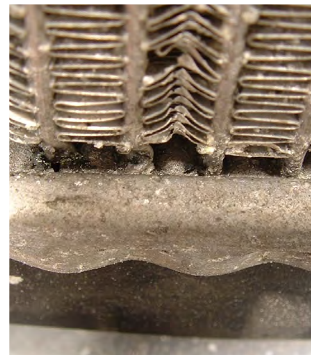
Fig. 1: Corrosion on the radiator
