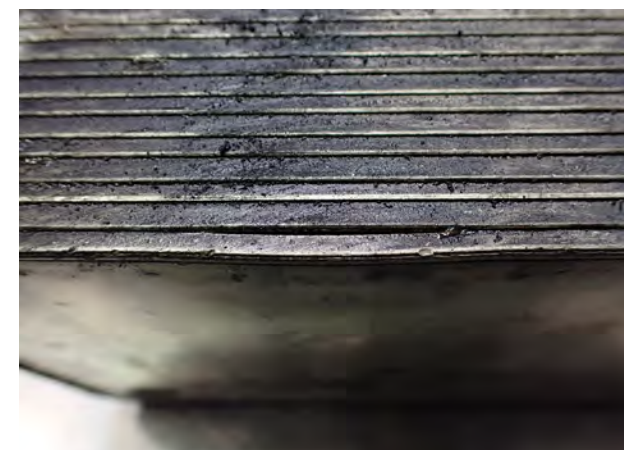
Fig. 2: Leaky oil cooler
