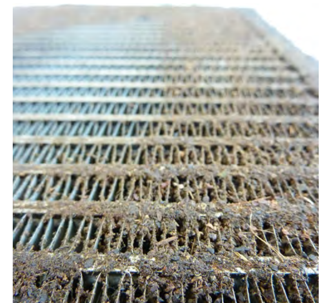
Fig. 2: Clogged evaporator
