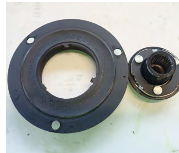
Fig. 1: Broken overload protection
