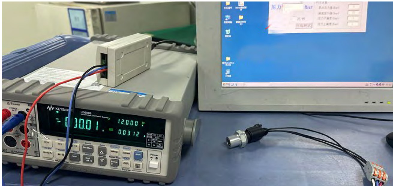
Fig. 4: Testing a pressure switch in the laboratory
