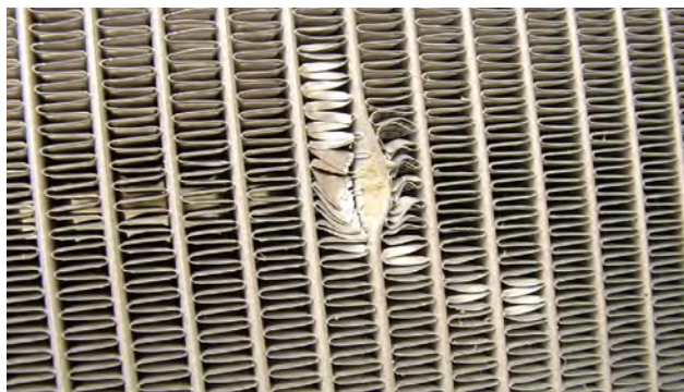
Fig. 3: Stone chipping on the radiator
