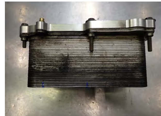
Fig. 1: Leaky oil cooler
