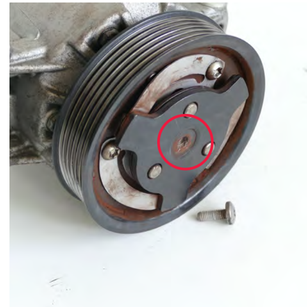
Fig. 1: Loosened central screw
