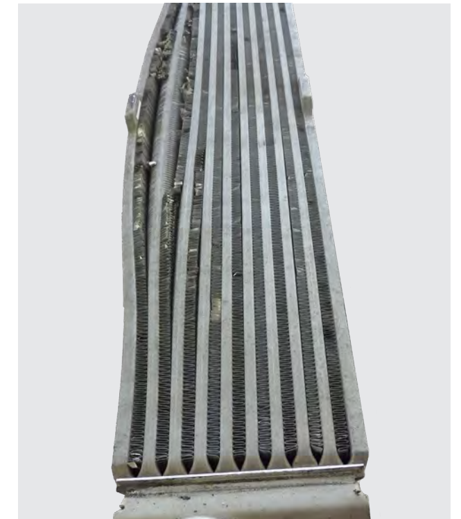
Fig. 2: Swollen charge air cooler
