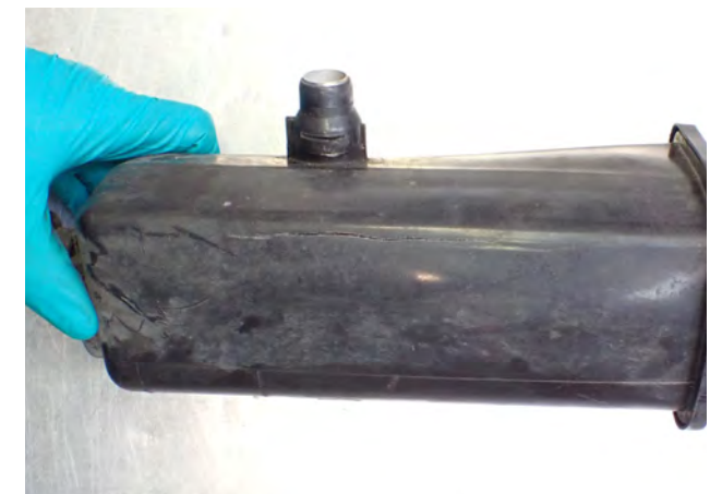
Fig. 2: Burst expansion tank
