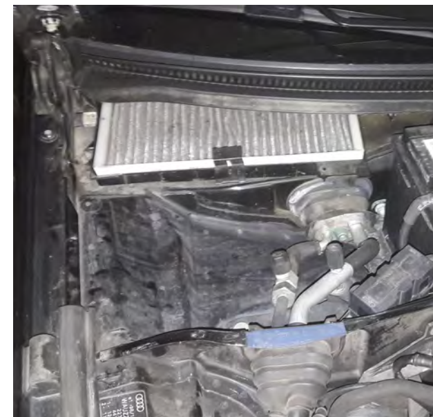
Fig. 1: Heavily soiled cabin filter
