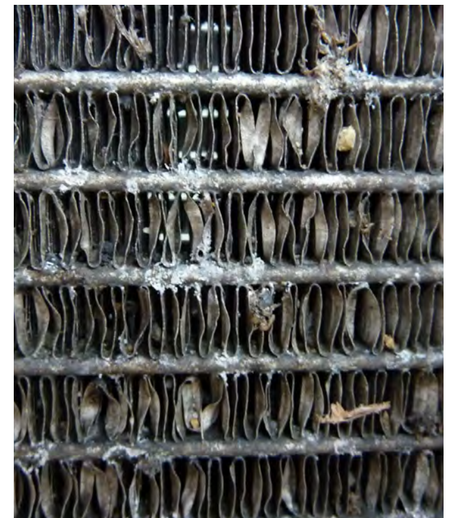
Fig. 2: Contaminants and deformed cooling fins
