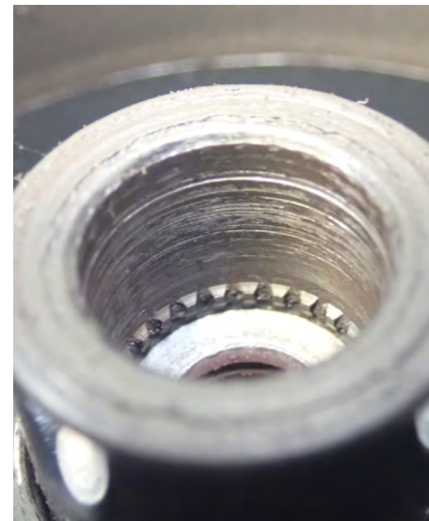
Fig. 3: Worn out teeth
