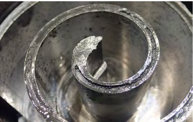
Fig. 2: Seal on front face of scroll destroyed
