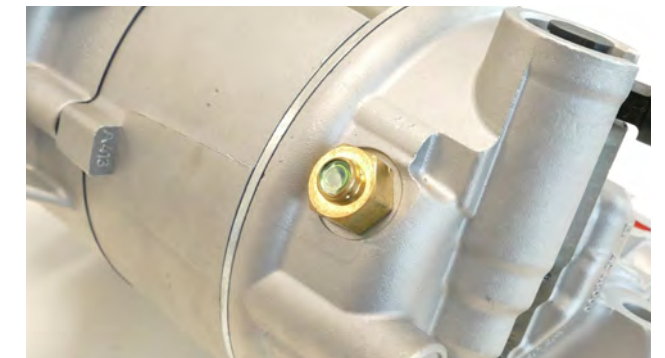
Fig. 2: Protective film indicates that valve has not activated
