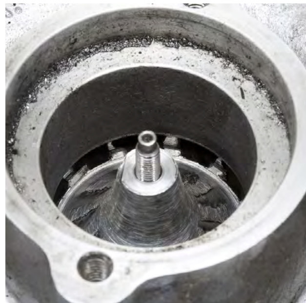
Fig. 2: Chips from turbo damage
