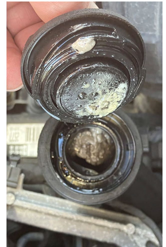
Fig. 3: Oil-in-water emulsion in the oil filler neck
