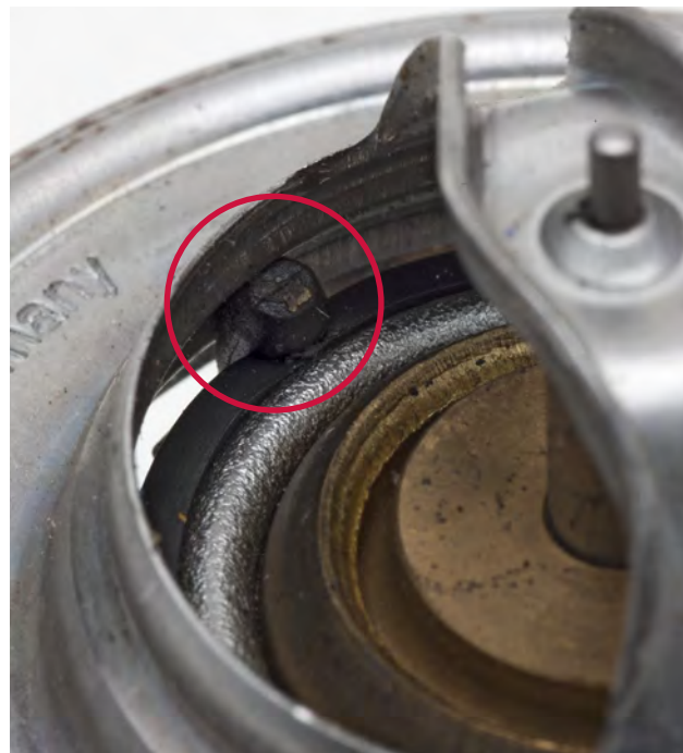
Fig. 1: Foreign object blocking the valve
