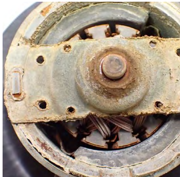
Fig. 1: Bearing damage to the fan motor
