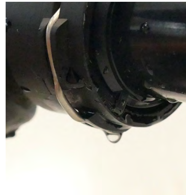
Fig. 1: Leaky O-ring
