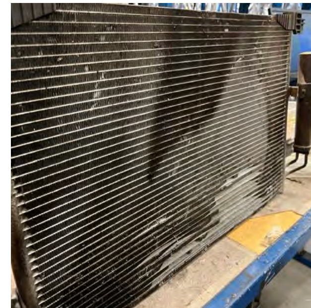
Fig. 1: Corrosion on the condenser
