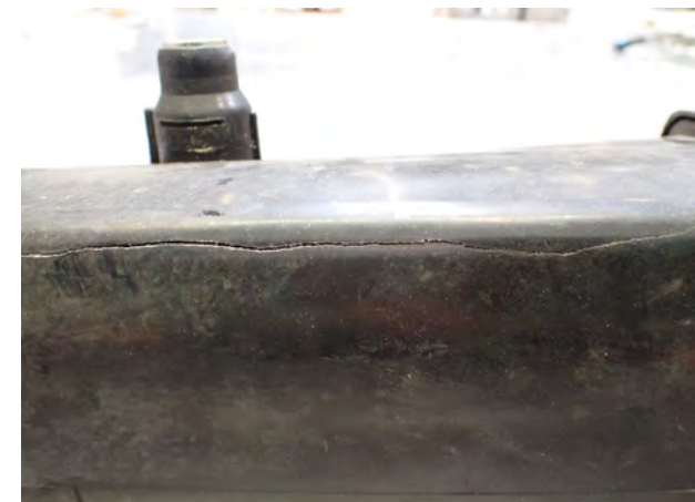
Fig. 1: Crack in the expansion tank
