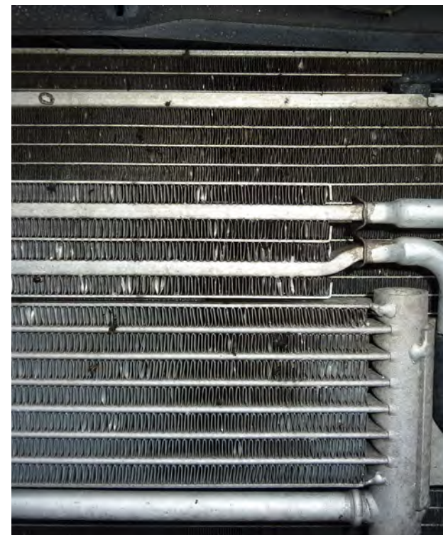
Fig. 1: Contamination on the radiator
