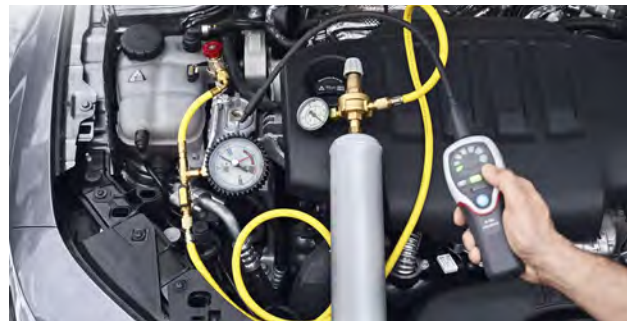
Fig. 1: Leak detection using forming gas
