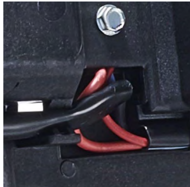
Fig. 2: Broken cable to fan control unit
