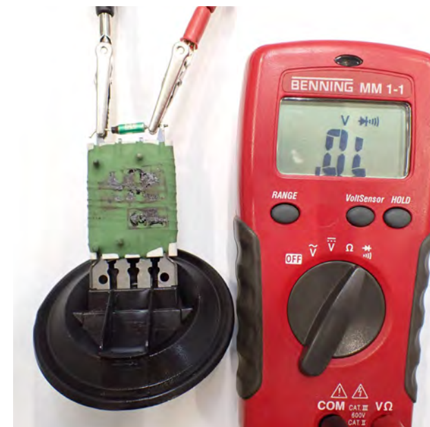
Fig. 1: Testing a burned-out controller
