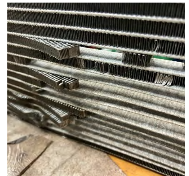
Fig. 2: Corroded cooling fins
