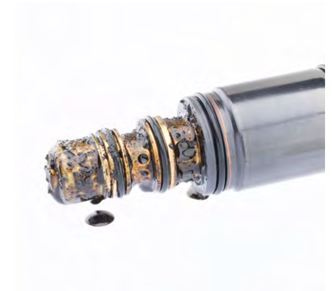
Fig. 4: Chips and black oil on the solenoid valve
