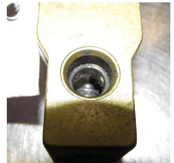
Fig. 2: Contaminants in the expansion valve
