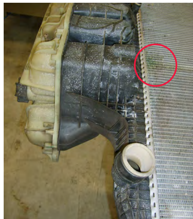
Fig. 1: Radiator appears to be leaking
