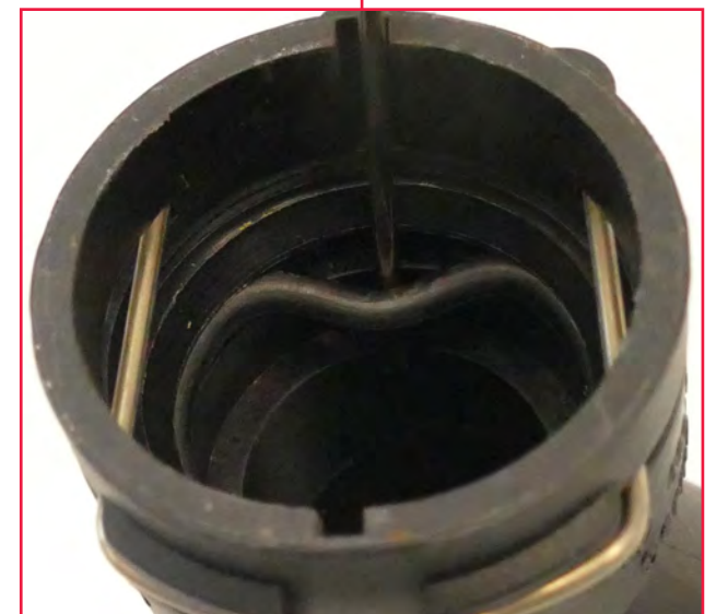
Fig. 3: Replace O-ring
