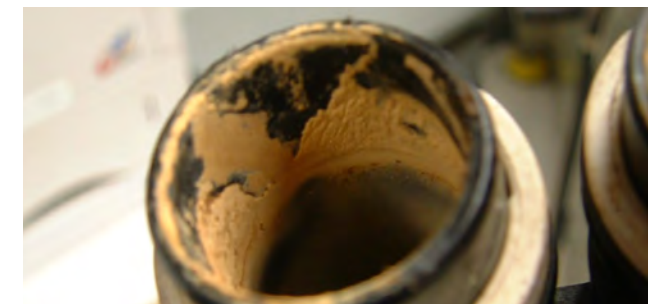
Fig. 3: Corrosion and deposits in the coolant circuit
