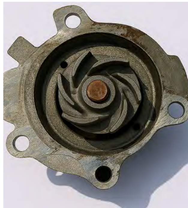
Fig. 2: Metal impeller detached from shaft
