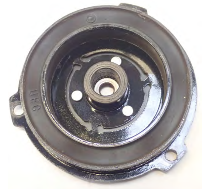
Fig. 2: Worn out teeth in the hub
