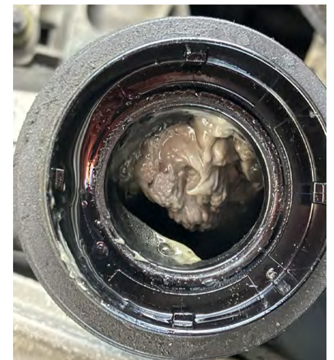
Fig. 3: Oil-in-water emulsion in the oil filler neck
