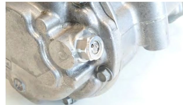
Fig. 1: Pressure-relief valve has activated
