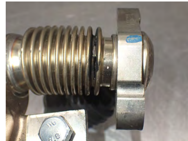
Fig. 1: Crack in the flexible pipe from the EGR cooler
