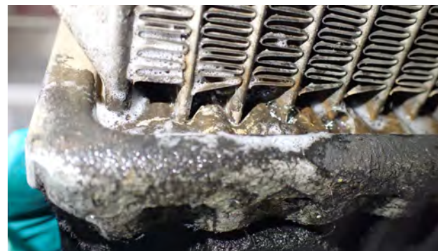
Fig. 4: Corrosion on the exterior of the radiator
