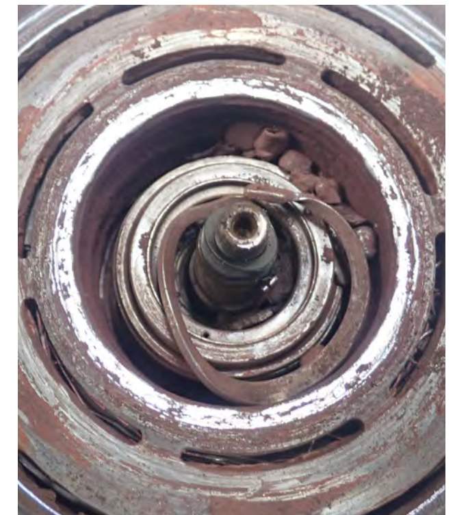
Fig. 2: Defective ball bearing
