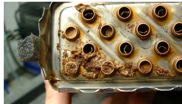
Fig. 2: Clogged heat exchanger
