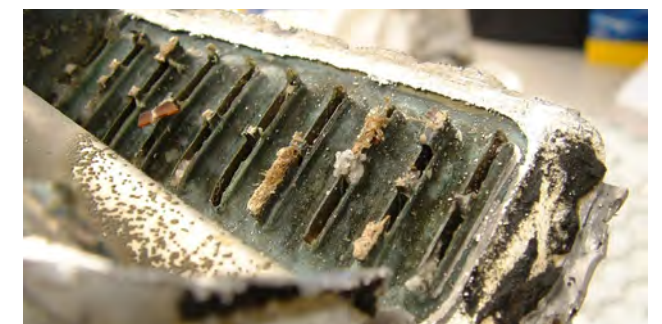
Fig. 2: Radiator blocked by sealant
