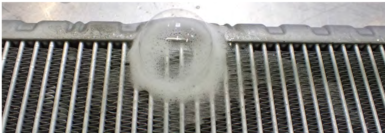
Fig. 3: Leaky evaporator
