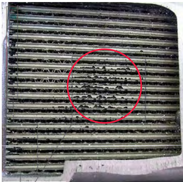
Fig. 1: Cavitation on the oil cooler tubes
